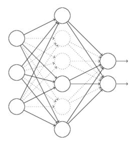
Figure 3. Fully connected neural network after applying dropout on the hidden layer.
